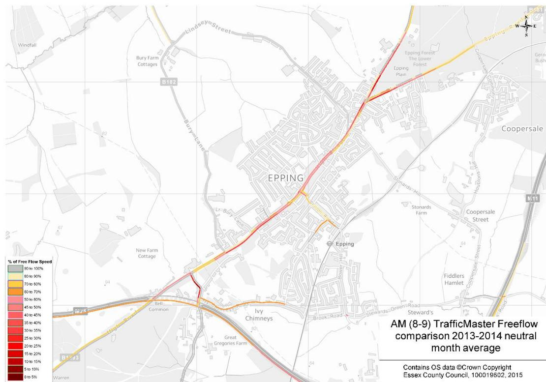
Figure 2.2: Peak hour speed as a percentage of free flow speed – AM Peak
