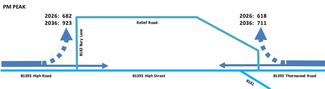
Figure 4.3 below illustrates the difference in flows along the B1393 between the existing network and the modelled network incorporating a western relief road. This effectively represents the total diverted traffic flow (background flow and development traffic)
