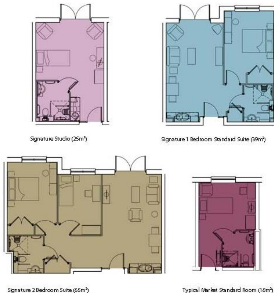
Figure 3: Typical Signature Senior Lifestyle bedroom and apartment layouts compared to a standard care home bedroom
