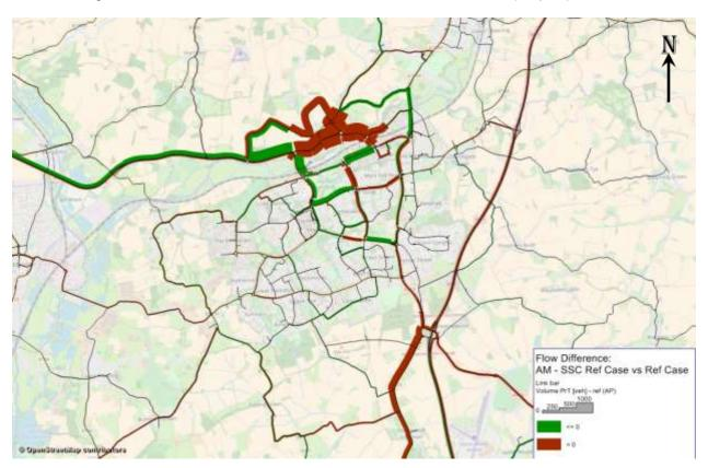
Figure 4-2: Flow Differences Reference Case with SSC v. – Reference Case (AM peak) S1 vs E1
