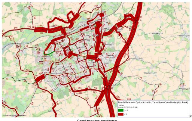
Figure 3-2 Flow Differences 2033 Reference Case vs 2014 Base Year - AM
